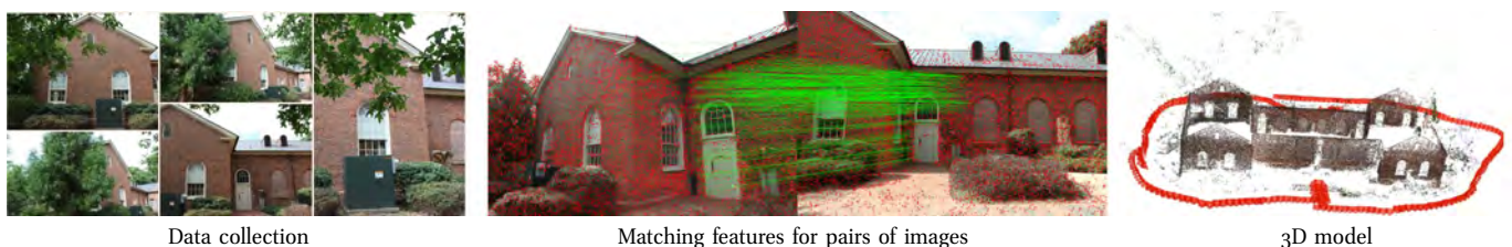
Figure 1: Structure from Motion pipeline. In the final 3D model the cameras are in red and the triangulated points are in black. The reconstruction was done with COLMAP [7] using their data set person-hall .
